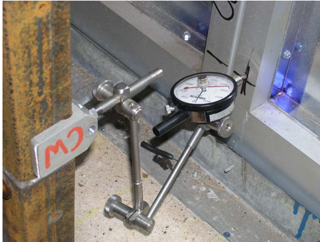
Figure 3. Strain gauges for measuring inter-story drift
