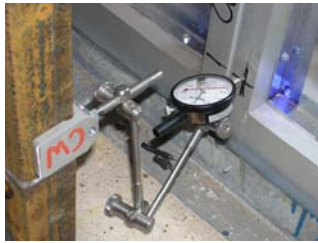
Figure 3. Strain gauges for measuring inter-story drift
