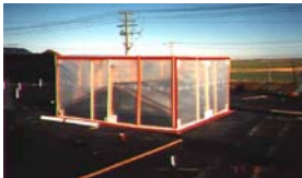
A chamber is created using polyethylene and a simple wood frame (Figure 2), a smoke device is released, or generated using theatrical foggers, while air from a fan depressurizes or pressurizes depending on the configuration.
